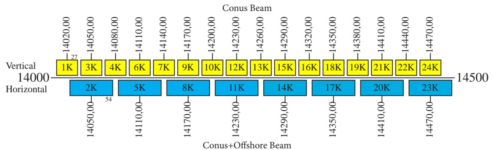
Cross-strapping : Ku-Band transponders 17 and 23 can cross-strapp to C-Band transponders 18 and 24.
